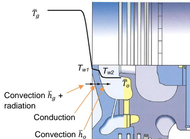
Figure 2: Combined heat transfer in piston
