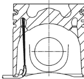
Figure 1: Piston jet cooling principle [1]
