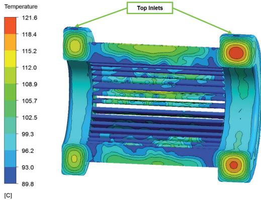
Figure 16: Temperature Map (4L/min in Rotor Shaft) Viewed in Section
