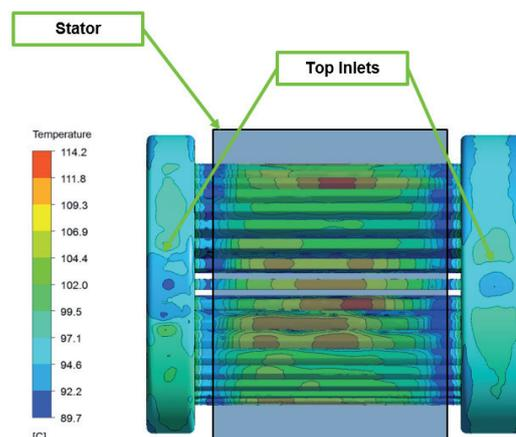
Figure 15: Temperature Map (4L/min in Rotor Shaft) Viewed From Above
