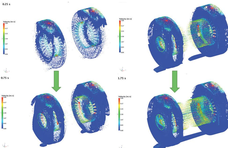
Figure 10: Development of Oil Flow (Without Air)
