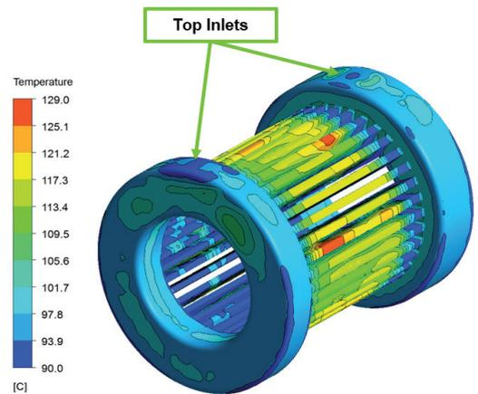
Figure 20: Temperature Map (2L/min in Rotor Shaft)
