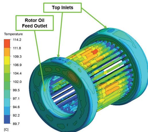
Figure 14: Temperature Map (4L/min in Rotor Shaft)
