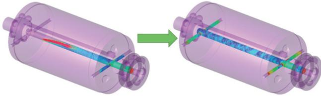
Figure 9: Oil Flow Through Rotor Shaft
