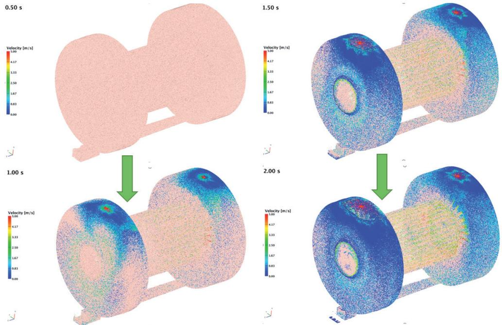
Figure 11: Development of Oil Flow (With Air)
