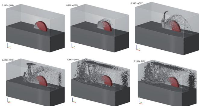
Figure 5: Correlation model of single gear in oil (6)
