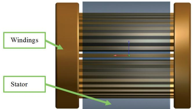
Figure 7: Stationary Components
