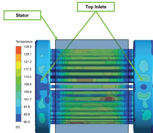
Figure 21: Temperature Map (2L/min in Rotor Shaft) Viewed From Above
