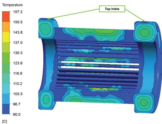
Figure 17: Temperature Map (6L/min in Rotor Shaft)
