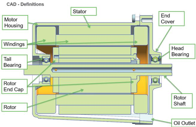
Figure 3: e-machine Design
