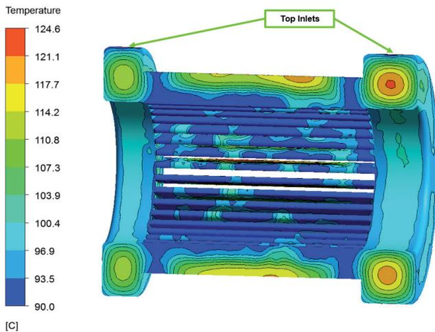
Figure 22: Temperature Map (2L/min in Rotor Shaft) Viewed in Section
