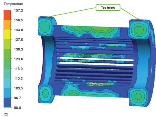
Figure 19: Temperature Map (6L/min in Rotor Shaft) Viewed in Section
