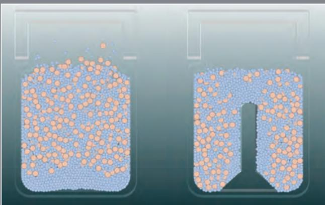
Container design to prevent segregation due to vibration during transportation
