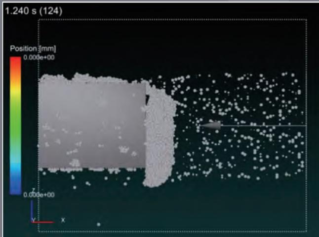
Snow Adhesion and Accumulation on a Wall
