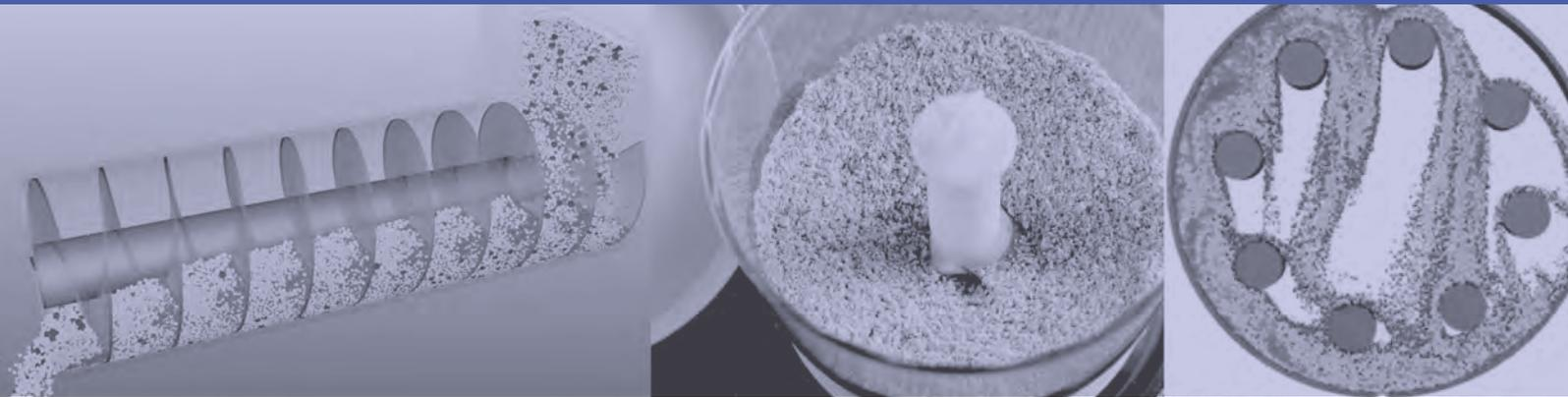
Granuleworks is a granular material simulation software based on the discrete element method (DEM) theory. It can be used for manufacturing processes using powders, powder processing, and design and improvement of powder equipment for various fields including food, pharmaceuticals, chemicals, transport equipment, and electronic materials. Granuleworks can easily simulate the phenomena of powder mixing, transport, filling, etc.
