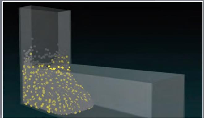
Concrete Flow Simulation with Aggregate
