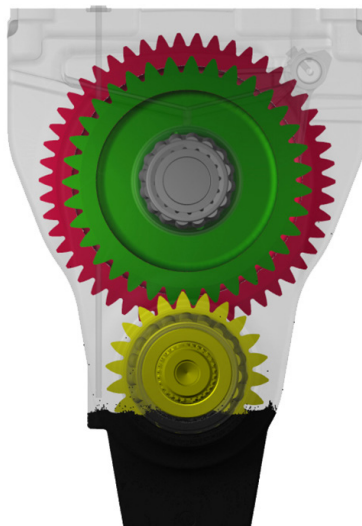
Figure 2 - MPS model of the speed reduction gear box with the initial oil volume at the bottom.
