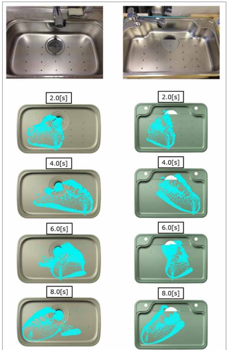
Fig. 4 - Water flow simulation for conventional type (left) and Niagara Flow Type (right)holes
